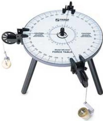
A force table is a physics lab apparatus that consists of a small table with a 360 degree circle printed on the top, along with 3 strings tied to a central ring. The strings go over pulleys and are attached to platforms, from which varying masses can be hung. The pulleys themselves can be moved to any angle along the outside of the circle, so that the center ring can be pulled in 3 different directions by 3 different masses.
