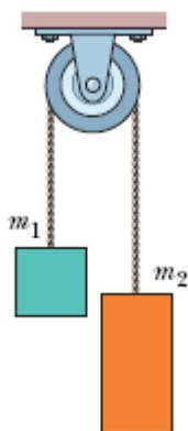
Each lab station is equipped with a *smart pulley* and a piece of string tied to two mass hangers. Different masses placed on each of the hangers will cause the system to accelerate at different rates.
