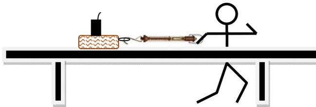
In this experiment, you will study the effects of various factors on the force of friction between a wooden block and the lab bench. Specifically, you will test the effects of surface area, speed, surface material, and normal force on the amount of force required to drag the block across the table at a constant speed.
